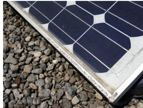
Soiling on bottom edge in proximity to the ground:
