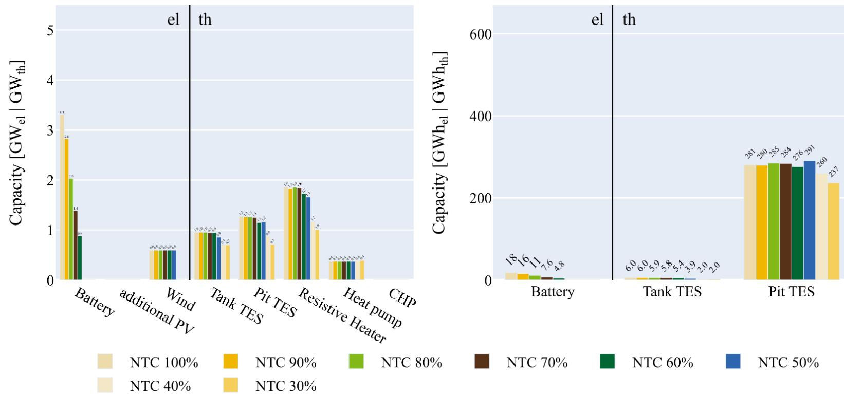
In winter, mostly efficient heat pumps are used. In summer, resistive heaters are used with heat pumps to exploit zero price hours
