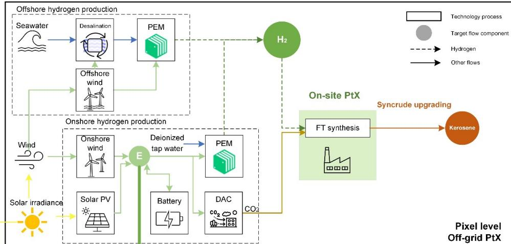
PtX fuel: PEM hydrogen, DAC-PEM-FT-SAF (kerosene)
